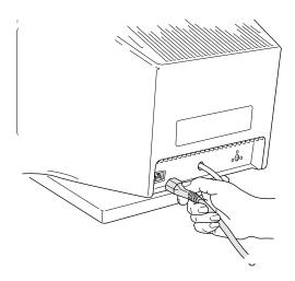
2 Plug the other end of the power cord into the power socket on the back of the computer.
